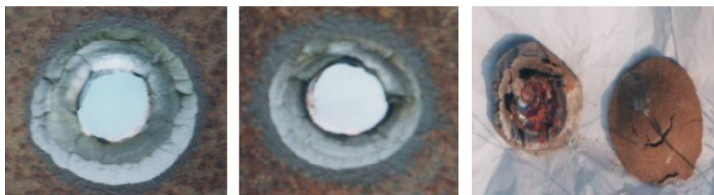
Figure 2.4 Penetration of a 2.54 cm Steel Plate (Wu, 2007)
