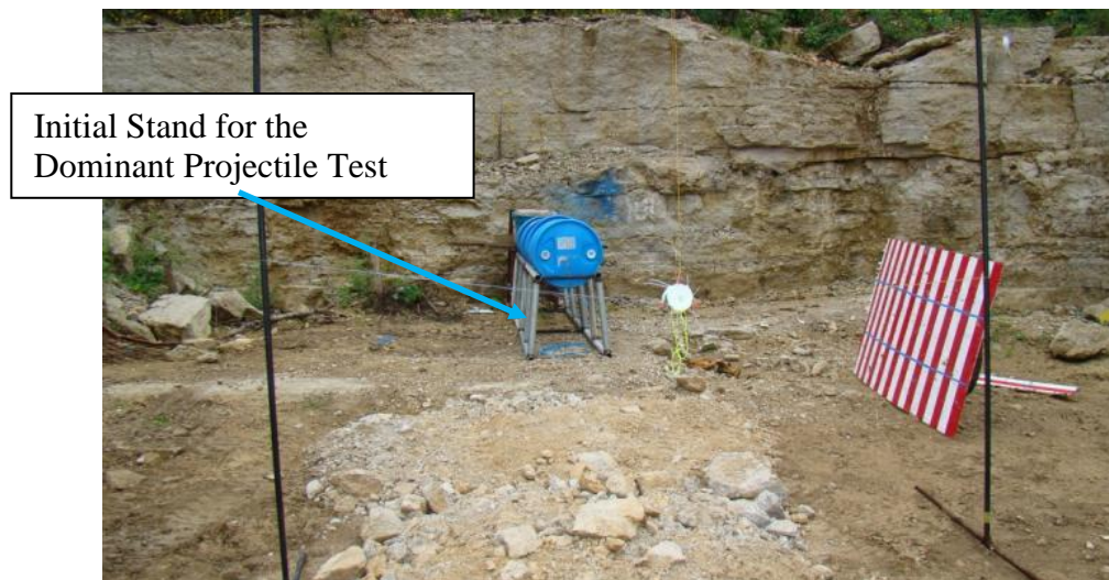
Figure 4.15 Initial Dominant Projectile Test Set-up
