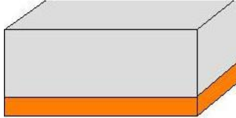
Figure 4.8 Open-Faced-Sandwich Gurney Equation Configuration
